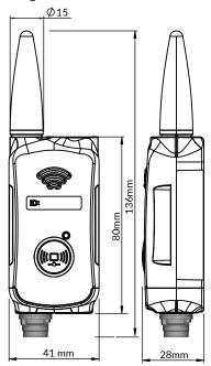
Designed to work with tek troniks D3 wireless base stations and is compatible with a full range of tek troniks Inteligent sensors.
